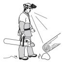
5 Take great care when cutting a tree that is under tension. A tree that is under tension may spring back to its normal position before or after being cut. If you position yourself incorrectly or make the cut in the wrong place the tree may hit you or the machine and cause you to lose control. Both situations can cause serious personal injury.
