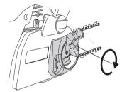
· Fold the knob back in to lock the tensioning.
