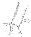
We recommend that you use a bar that is longer than the diameter of the tree, so that you can make the felling cut and directional cuts with single cutting strokes. See instructions under the heading Technical data section to find out which lengths of bar are recommended for your saw.
