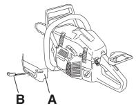
These reduce the flow of cooling air and prevent large amounts of snow from being sucked into the carburetor space.
