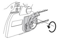
Adjust the tension on the chain by turning the wheel down
