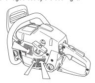
IMPORTANT! In order to maintain operation of the centrifugal cleaning system it must be regularly maintained. Clean the air intake to the starter, the fins on the flywheel, the space around the flywheel, inlet pipe and carburettor compartment.
