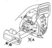
Fit the bar over the bar bolts. Place the bar in its rearmost position. Place the chain over the drive sprocket locate it in the groove on the bar. Begin on the top edge of the bar.
