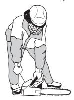
As the chain brake is still engaged the speed of the engine must be set to idling as soon as possible, this is achieved by quickly disengaging the throttle lock. This prevents unnecessary wear to the clutch, clutch drum and brake band.
