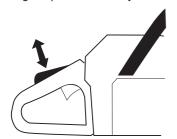
Check that the throttle control and throttle lockout move freely and that the return springs work properly.
