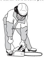
As the chain brake is still activated the engine must return to idling speed as soon as possible by disengaging the throttle latch in order to avoid unnecessery wear on the clutch assembly.
