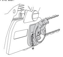
The chain is correctly tensioned when it does not sag from the underside of the bar, but can still be turned easily by hand. Hold up the bar tip and tighten the bar clutch by turning the knob clockwise.
