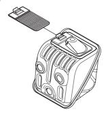
The muffler is designed to reduce the noise level and to direct the exhaust gases away from the operator. The exhaust gases are hot and can contain sparks, which may cause fire if directed against dry and combustible material.
