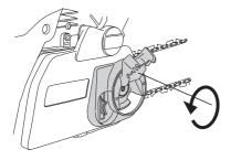
Adjust the tension on the chain by turning the wheel down
