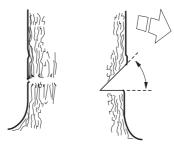
The line where the two cuts meet is called the directional cut line. This line should be perfectly horizontal and at right angles (90°) to the chosen felling direction.
