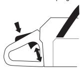
Start the chain saw and apply full throttle. Release the throttle control and check that the chain stops and remains stationary. If the chain rotates when the throttle control is in the idle position you should check the carburetor idle adjustment.
