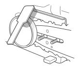
Regularly check that the brake band is at least 0.6 mm (0,024 inch) thick at its thinnest point.
