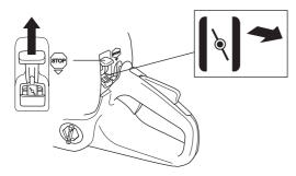
**Start throttle:** The correct choke/start throttle setting is obtained by moving the control to the choke position.
