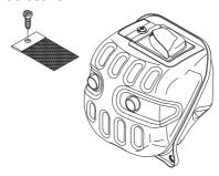
The muffler is designed to reduce the noise level and to direct the exhaust gases away from the operator. The exhaust gases are hot and can contain sparks, which may cause fire if directed against dry and combustible material.
