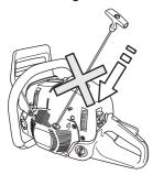
Note! Pull the front hand guard towards the front handle. The chain brake is now disengaged. Your saw is ready for use.
