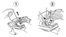
Undo the screw in the centre of the pulley and remove the pulley. Insert and fasten a new starter cord to the pulley. Wind approx. 3 turns of the starter cord onto the pulley. Connect the pulley to the recoil spring so that the end of the spring engages in the pulley. Fit the screw in the center of the pulley. Insert the starter cord through the hole in the starter housing and the starter handle.
