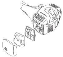
An oiled foam plastic filter (available as an accessory) must be used if the machine is operated in extremely dusty conditions. See instructions under the heading Oiling the air filter.
