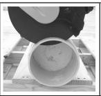
Position machine at top of plastic pipe to begin cutting through the pipe wall.
