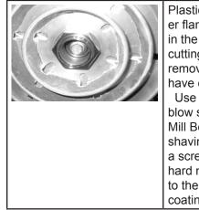
Plastic debris from a smaller flange often lodges itself in the bigger flange during cutting. This can easily be removed once the flanges have cooled down. Use compressed air to blow shavings from Speed-Mill Bowl. DO NOT scrap shavings from bowl using a screwdriver or any other hard metallic tool. Damage to the bowls or abrasive coating could occur.
