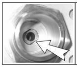
Mount the SpeedMill Bowl Assembly. Align the slot in the SpeedMill Hub with the face of the shaft. Make sure the flange face of the SpeedMill Hub contacts the face of the blade.
