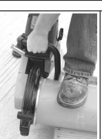
Align proper SpeedMill Bowl with end of pipe, and move toward the pipe so that the pipe is slightly beveled. Note: The bevel required is usually quite small, so do not remove excessive pipe material.
