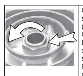
Change the mounted bowl sizes if desired. Turn the 2" (50.8mm) hub nut Counter-Clockwise to remove. Lift off the smaller bowls, and configure the bowl / hub assembly as desired. Example: 6" and 8" bowl combination is popular. ALWAYS mount the 8" bowl, it may shield operator in case of blade breakage.
