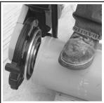
Bevel Pipe: Position SpeedMill Bowl near end of pipe to be beveled. Accelerate power cutter to full throttle.
