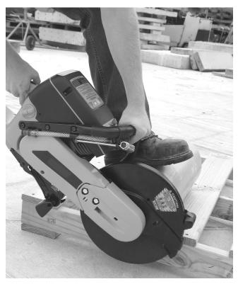
**HOLD MACHINE ONLY** at front and rear handles, as shown in the above photo.
