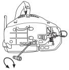
The oil tank should become nearly empty by time fuel is used up. Be sure to refill the oil tank every time when refueling the saw.
