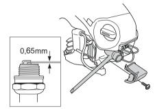
Note! Always use the recommended spark plug type! Use of the wrong spark plug can damage the piston/cylinder. Check that the spark plug is fitted with a suppressor.
