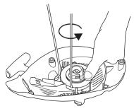
Undo the screw in the centre of the pulley and remove the pulley. Insert and fasten a new starter cord to the pulley. Wind approx. 3 turns of the starter cord onto the pulley. Connect the pulley to the recoil spring so that the end of the spring engages in the pulley. Fit the screw in the centre of the pulley. Insert the starter cord through the hole in the starter housing and the starter handle. Make a secure knot in the end of the starter cord.
