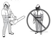
Always hold the saw with both hands. The right hand should be on the top handle, and the left hand on the front handle. All people, whether right or left handed, should use this grip. Use a firm grip with thumbs and fingers encircling the chain saw handles.
