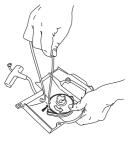
Undo the screw in the centre of the pulley and remove the pulley. Insert and fasten a new starter cord to the pulley.
