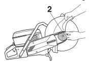
Position the belt guard and secure the cutting head together with the belt guard. Tighten both bolts (4) by hand.
