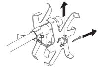
Remove the tine unit from the angle gear's output axle.
