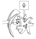
CAUTION! The gear housing must not be filled completely with grease. The grease expands as the machine heats up during operation. If the gear housing was completely filled with grease it could damage the seals and lead to leakage of grease.
