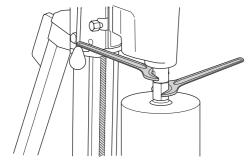
Before the machine is started, carefully check that the new bit is firmly attached.
