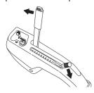
2 Release the clip on the front hood and lift off the fender.
