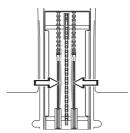
If necessary, the wires can be adjusted by tightening the adjuster nuts on each side of the steering collar. Do not over tighten the cables; they should only be drawn in towards the steering collar.
