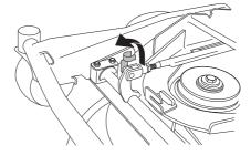
3 Remove the bolt so the track rod is released in one end.
