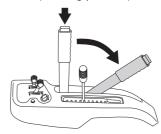
The lever can also be used to temporarily regulate the cutting height, e.g. for a small mound in the lawn.
