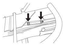
3 Screw out (extend) the stay to raise the rear edge of the
