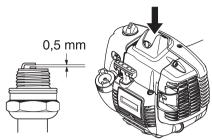
**CAUTION!** Always use the recommended spark plug type! Use of the wrong spark plug can damage the piston/cylinder. Check that the spark plug is fitted with a suppressor.
