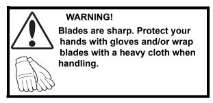
Bent or cracked blades or blades with large nicks should be replaced.
