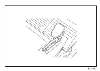
Raise the mower deck with the lifting pedal
