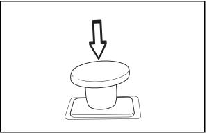
Disengage the mower deck
