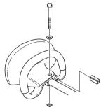
3 Now make a final adjustment to give yourself a comfortable working position. Tighten the screw. CAUTION! The loop handle and hand guard must not be fitted behind the arrow marked on the shaft.
