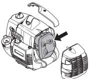
Some mufflers are equipped with a special spark arrestor screen. If your machine has this type of muffler, you should clean the screen at least once a week. This is best done with a wire brush.
