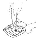
CAUTION! Check that the pulley can be turned an additional 1/2 turn when the starter cord is pulled all the way out.
