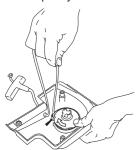
CAUTION! Check that the pulley can be turned at least a further 1/2 turn when the starter cord is pulled all the way out.
