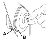
The shaft can be locked using a screwdriver, steel pin or the like. This is slid in as far as possible. The blade is tightened clockwise.
