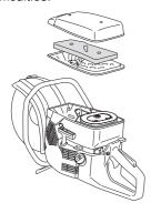
If the machine is low on power, difficult to start or runs poorly at idle speed: always check the spark plug first before taking any further action. If the spark plug is dirty, clean it and check that the electrode gap is 0.5 mm. The spark plug should be replaced after about a month in operation or earlier if necessary.
