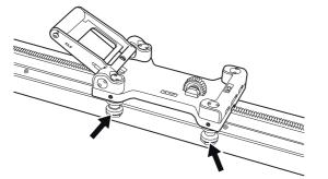
Start by loosening the marked nuts (1) with the supplied special tool. Now loosen the two stop screws (2). When these are loose, adjust the guide wheels (3) against the rail by turning them towards the rail so the play is taken up. Hold the guide wheels and screw in the stop screw. Now screw on the nuts to secure the guide wheels in the new position.
