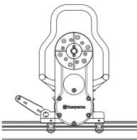
2 To secure the saw, lift the locking handle towards the saw until the handle locks.
