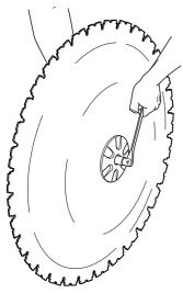
4 Hang the blade with the blade flange and blade flange hub fitted on the cutting arm (blade is not shown in the figure).
