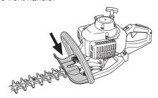
Check that the hand guard is fitted correctly.
