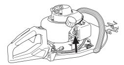
**Choke:** Set the choke control in the choke position.
