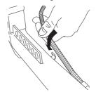
Put on the harness and hang the machine from the support hook. Now make a final adjustment so that the machine is in a comfortable working position when it hangs from the harness. Tighten the knob.
