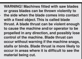
Avoid cutting with the area of the blade between the 12 o'clock and 3 o'clock positions. Because of the speed of rotation of the blade, blade thrust can occur if you attempt to cut thick stems with this area of the blade.
