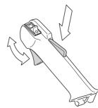
See instructions under the heading Start. Start the machine and apply full throttle. Release the throttle and check that the cutting attachment stops and remains at a standstill. If the cutting attachment rotates with the throttle in the idle position then the carburettor idle setting must be checked. See instructions under the heading Maintenance.
