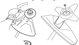
The nylon lining inside the locking nut must not be so worn that you can turn it by hand. The lining should offer a resistance of at least 1.5 Nm. The nut should be replaced after it has been put on approx. 10 times.
