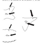
Check that the support flange is not cracked due to fatigue or due to being tightened too much. Discard the support flange if it is cracked.
