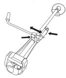
Now make a final adjustment, with the machine hanging from the harness, to obtain the most comfortable working position. Tighten the screws.
