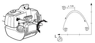
CAUTION! If the cutting attachment rotates when the engine is idling the idle adjustment screw T should be turned anticlockwise until the cutting attachment stops.
