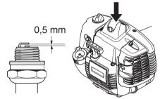
**CAUTION!** Always use the recommended spark plug type! Use of the wrong spark plug can damage the piston/ cylinder.
