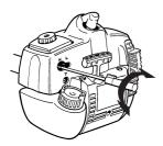
Apply full throttle and turn the high speed jet H very slowly clockwise until the engine slows down. Then turn the high speed jet H very slowly anticlockwise until the engine starts to run unevenly. Now turn the high speed jet H slowly clockwise a little way until the engine runs smoothly.
