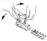
Press the cutting head against the ground or some other solid object until the desired angle has been obtained.
