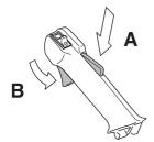
Make sure the throttle control is locked at the idle setting when the throttle lock is released.
