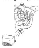
Some mufflers are equipped with a special spark arrestor mesh. If your machine has this type of muffler, you should clean the mesh at least once a week. This is best done with a wire brush.
