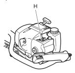
Apply full throttle and turn the high speed jet H very slowly clockwise until the engine slows down. Then turn the high speed jet H very slowly anticlockwise until the engine starts to run unevenly. Now turn the high speed jet H slowly clockwise a little way until the engine runs smoothly. Note that the engine should not be under load when the high speed jet is adjusted.
