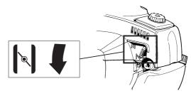
Hold the body of the machine on the ground using your left hand (CAUTION! Not with your foot!). Grip the starter handle, slowly pull out the cord with your right hand until you feel some resistance (the starter pawls grip), now quickly and powerfully pull the cord. **Never wrap the starter cord around your hand**
