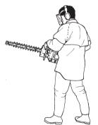
Make sure that your hands and feet do not come near the cutting attachment when the engine is running.
