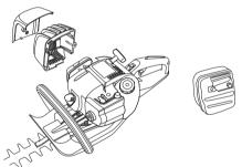
Some mufflers are equipped with a special spark arrestor mesh. If your machine has this type of muffler, you should clean the mesh at least once a week. This is best done with a wire brush.
