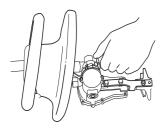
Press the cutting head against the ground or some other solid object until the desired angle has been obtained.
