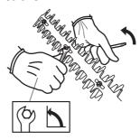
The edges of the blades are too hard to be filed. Dull blades should be sharpened using a grinder.
