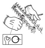
When the blades are correctly adjusted the play between the blades should be 0,2–0,4 mm, measured at the screws.
