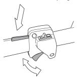
See instructions under the heading Start. Start the machine and apply full throttle. Release the throttle and check that the cutting attachment stops and remains at a standstill. If the cutting attachment rotates with the throttle in the idle position then the carburettor idle setting must be checked. See instructions under the heading Maintenance.
