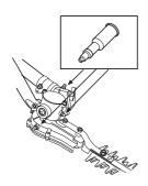
The grease in the bevel gear does not normally need to be changed except if repairs are carried out.
