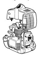
Some mufflers are equipped with a special spark arrestor mesh. If your machine has this type of muffler, you should clean the mesh at least once a week. This is best done with a wire brush.
