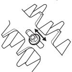
· Replace the blades if they are bent or damaged.
