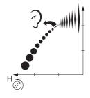
Note that the engine should not be under load when you adjust the high speed jet H. You should therefore remove the cutting attachment, nut, support flange and drive disc before adjusting the high speed jet H.
