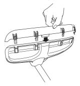
The guard extension is removed easily using the spark plug spanner, see illustration.
