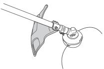
Check that the guard is undamaged and not cracked. Replace the guard if it has been exposed to impact or is cracked.
