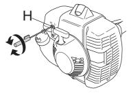
Note that the engine should be loaded when you adjust the high speed jet H. You should therefore fit the trimmer head T35 (2.7 mm cord) before adjusting the high speed jet. The cord length should be standard, i.e. to the knife on the trimmer guard.
