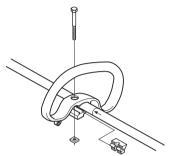
Slide the spacer into the slot in the loop handle. Fit the nut and screw. Tighten.
