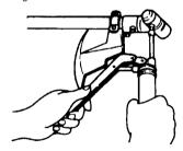
Remove the drive disc or the side bolt in the gear cae before installing new grease to arrange for old grease to exit.
