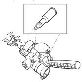
CAUTION! The gear housing must not be filled completely with grease. The grease expands as the machine heats up during operation. If the gear housing was completely filled with grease it could damage the seals and lead to leakage of grease.
