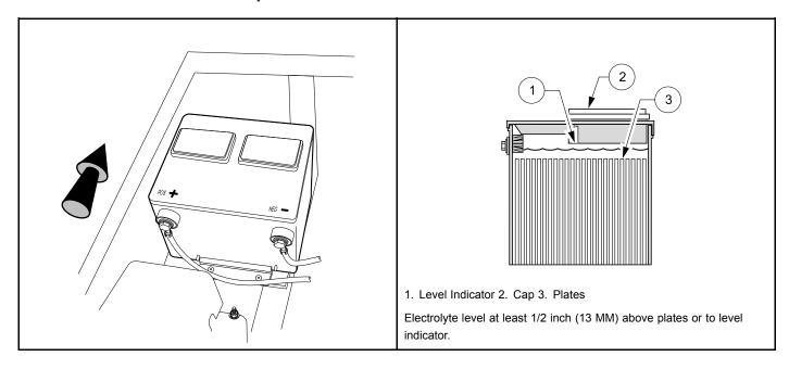
222 Figure 37 Battery Figure 38 Battery Electrolyte Level
