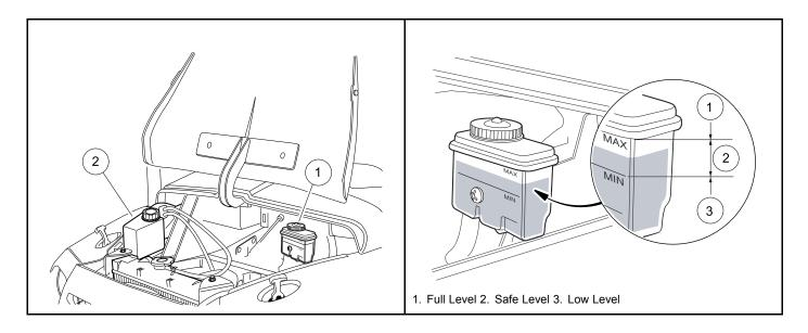
Figure 17 Brake Fluid and Coolant Access (diesel vehicle shown)
