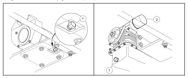
Figure 21 Engine Oil Drain Plug and Pan – Gasoline Vehicles
