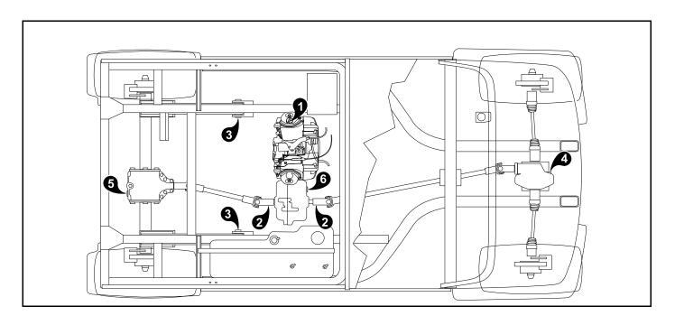
Figure 15 Lubrication Points – Gasoline Vehicles
