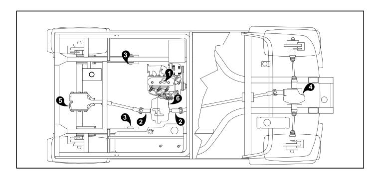
Figure 16 Lubrication Points - Diesel Vehicles
