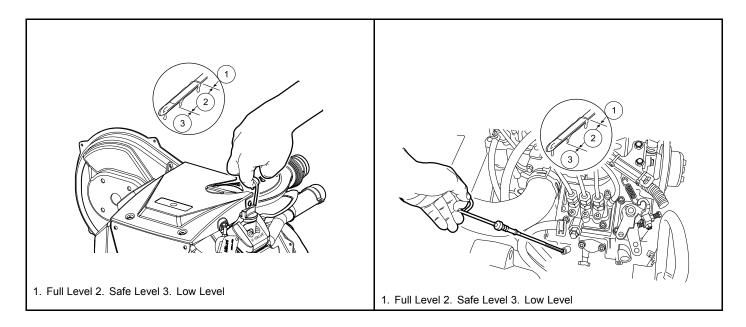
Figure 19 Engine Oil Level Check – Kawasaki Gasoline Vehicles
