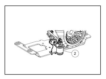
Figure 23 Replace Engine Oil Filter – Kawasaki Gasoline Vehicles
