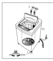
If the washer is installed on an unsuitable floor, it could make considerable noise, vibrate and cause a malfunction. If washer is not level, adjust the front leg(A) up or down for horizontal setting.
