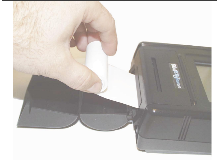
Figure 3-5. ICE 5500 printer paper installation
