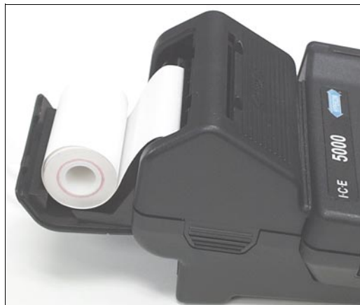
Figure 3-3. ICE 5000 Printer paper installation complete
