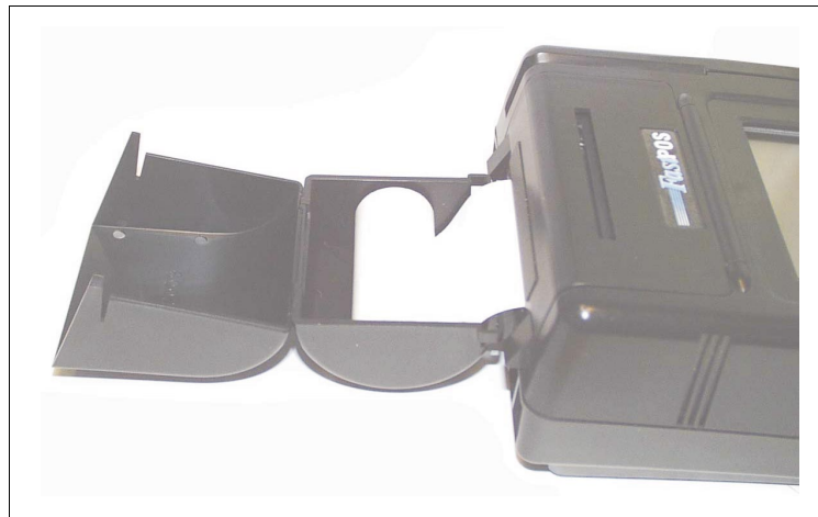
Figure 3-6. ICE 5500 Printer paper installation complete
