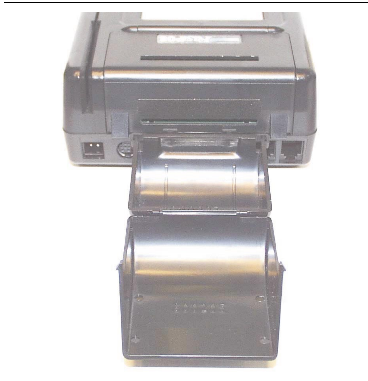
Figure 3-4. ICE 5500 printer paper door open
