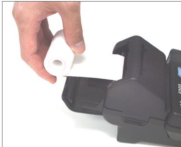
Figure 3-2. ICE 5000 printer paper installation
