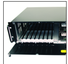
Eight slots for plug-in, hot-swappable port processors
