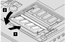
8. Replace the memory slot cover over the memory slot, aligning the back side of the cover first; then tighten the screw.
