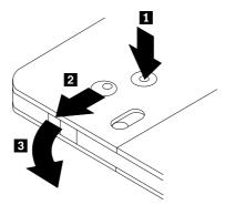
Using the tip of a ball point pen, push and break the lock pin tab 1. To remove the disc, use a ball point pen to push down on the cartridge lid lock 2 and pull the cartridge lid 3 out to eject the disc. With the cartridge lid
