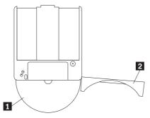
To return the disc to the cartridge, align the label side of the disc **1** with the DVD-RAM cartridge label side. Insert the disc, and close the cartridge lid **2**. A clicking sound will ensure that the lid door is closed.
