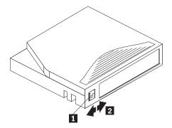
The front of the cartridge has an orange write-protect switch 1 to prevent accidental erasure. Slide the switch to the right to write-protect 2 or to the left to enable writing.
