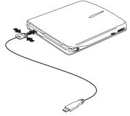
Make sure that the metal plate on the smaller connector is facing up when you plug it into the USB connector on the CD-ROM drive.
