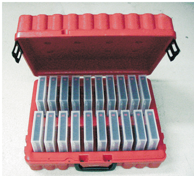
Figure 13. Tape cartridges in a Turtlecase
