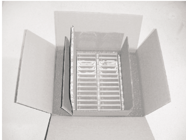
Figure 14. Double-boxing tape cartridges for shipping
