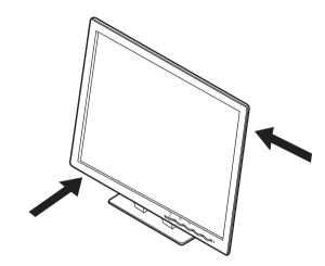
3. Before using your monitor for the first time, remove the clear protective film from the front of the screen.
