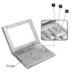
The volume indicator appears on the screen for a few seconds when you press one of these buttons. For more details on volume control, see the *Online User's Guide*.
