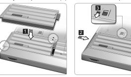
Secure the battery pack by sliding the battery-pack latch to the lock position (3).
